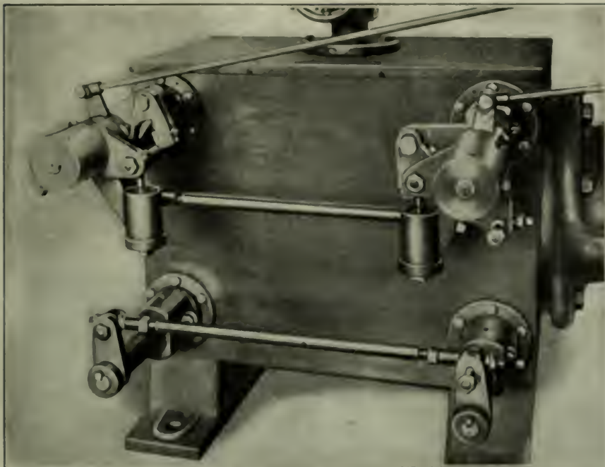
FIG. 2. NEAR VIEW OF VALVE GEAR
